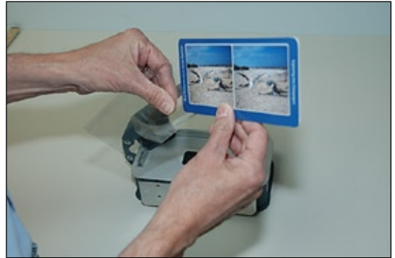
Remove the protective film from both sides, inspect and remove any stray glue. Insert finished card into the transparent sleeve.
