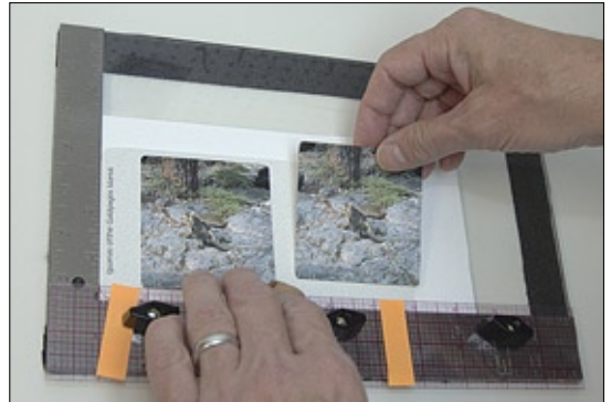
After placing clean paper, and the fully glued front and back card on the frame, roughly position each chip into position.
