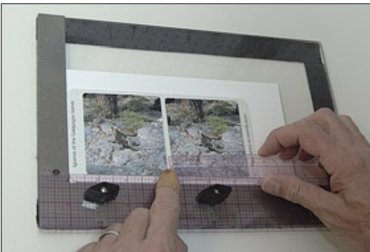
Set the center spacing so there is about 3 inches between the near points. Use the center of the card as the middle.
