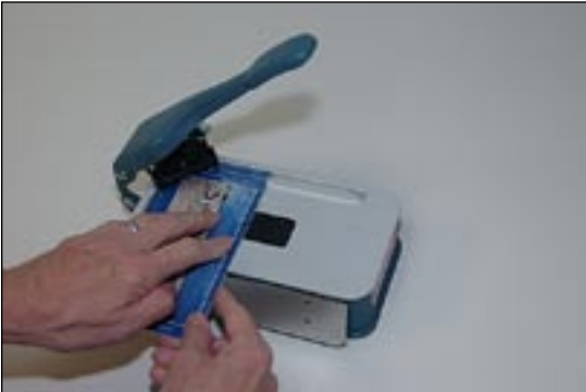
Round the corners to finish the card. The handheld rounders work, but are harder to use and won't last as long.
