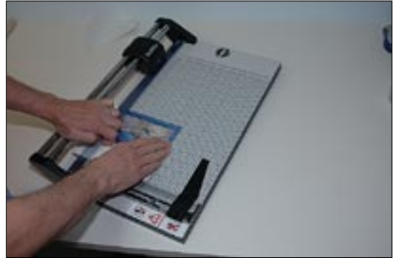
Trim each of the four edges to make the card the correct size. Only cut by pulling the blade toward you.
